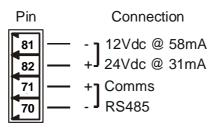
Warning: If the power/communication connections are reversed, the remote station may become faulty.
