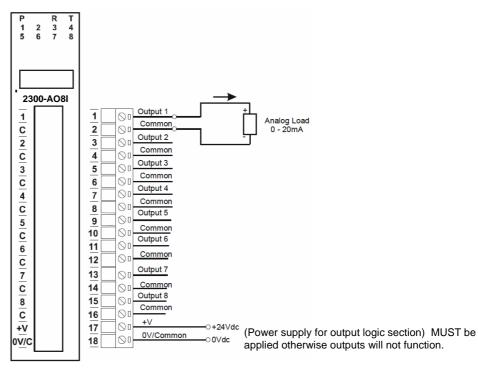
Note: Logic power output (terminals 17 & 18) range 24Vdc. The logic power supply output must be isolated and completely separate to the power supply that powers the 2300-AO8I on terminals 81 & 82. Failure to do so will cause the comms to stop.
