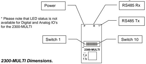
The 2300-MULTI enclosure is shown below. The station clips directly onto an industry standard DIN rail. Field wiring is on the top of the station via a separate plug in connector. The station power and RS485 communications wiring are on a separate plug in connector on the side of the housing.
