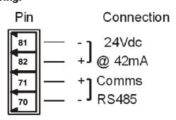
Warning: If the power/communication connections are reversed, the remote station may become faulty.
