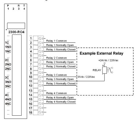
Note: Relay output is typically factory set to hold it's last state when comms is lost. A relay that is set to "on" by MicroScan can be set to automatically relax after comms fail, by setting the "Watchdog Timer". Please refer to MicroScan Help. Search for "Watchdog".
