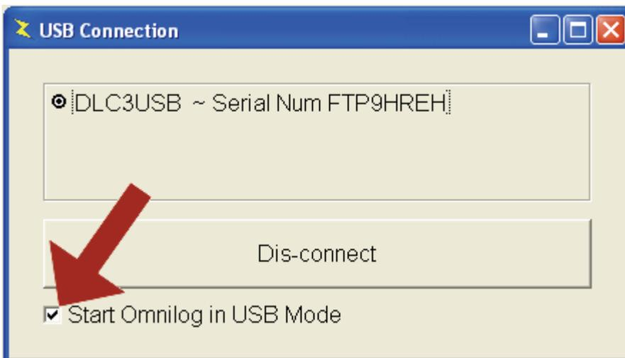
All TruTrack USB cables are based on the [Future Technology Devices International](#) USB chipset. This chipset is widely used for USB to RS232 Serial converter cables. USB to RS232 Serial converter cables, using this chipset, can now be used to connect TruTrack download cables to OmniLog without the need for a Virtual Com Port driver.
