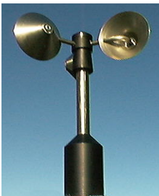
Wind Speed (3 cup Anemometer)
