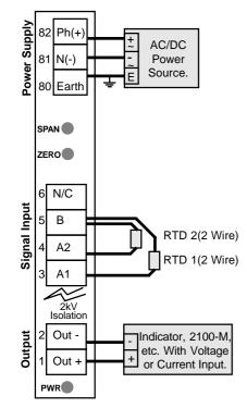
Note. All examples on RTD1 Sensor Break output will drive upscale & on RTD2 Sensor Break output will drive Downscale.
